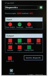
The **NEW** Diagnostics screen provides instant access to test the oven's inputs and outputs including the elements, fan, steam, damper, light and door catch for faster problem indentification and resolution.
